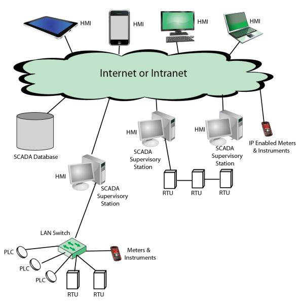
Figure C6.1 SCADA Example
